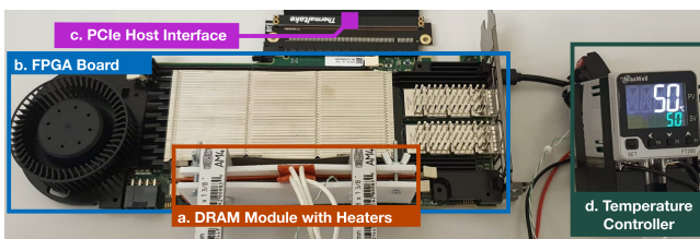
Fig. 2: SoftMC Infrastructure: (a) DRAM module under test clamped with heater pads, (b) Xilinx Alveo U200 FPGA board [154], programmed with a DDR4 version of SoftMC [38], (c) PCIe connection to the host machine, and (d) temperature controller.
