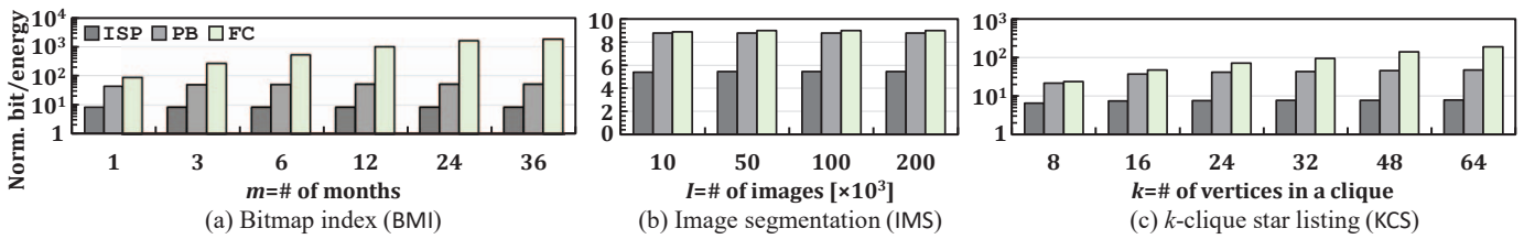
Figure 18: Energy-efficiency comparison of four computing platforms on three real-world workloads. Normalized to OSP (Outside-storage processing). Y-axis represents number of bits computed per unit of energy in log-scale.
